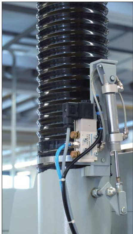
Mist Extraction Safety Flap Device (courtesy of Kraft & Bauer)
